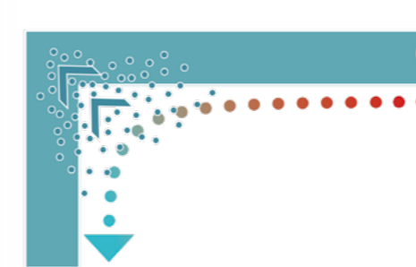
If the air is warmer than the enveloping surfaces it cools down on them. Moisture in the air condenses on and penetrates the walls.
